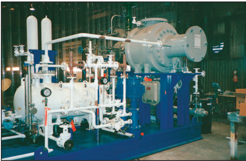
■ TDE typically uses Mafi-Trench turboexpanders on its cryogenic packages.
